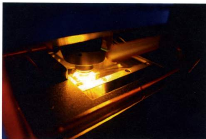
Figure 2 – The LODE LA-ICP-MS ablation cell (NWR 193)
